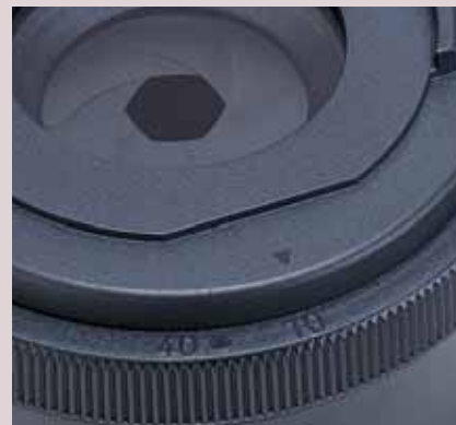
Field diaphragm with position guide markings
